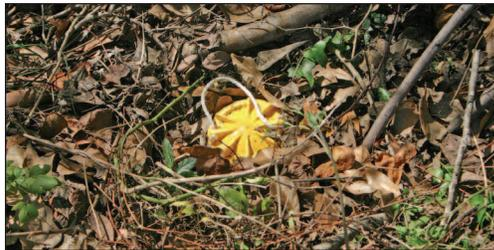
... and this is now. Seismic crews in the 1930s faced remote locations that meant difficult work. Today, geophysical crews can rely on plenty of technological advances (right); however, the wave of the future (no pun intended) may be found in cable-free land nodes (above), where a single channel P-wave sensor provides continuous recording from a single point receiver station.
