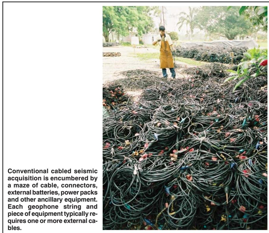
**Conventional cabled seismic acquisition is encumbered by a maze of cable, connectors, external batteries, power packs and other ancillary equipment. Each geophone string and piece of equipment typically requires one or more external cables.**
