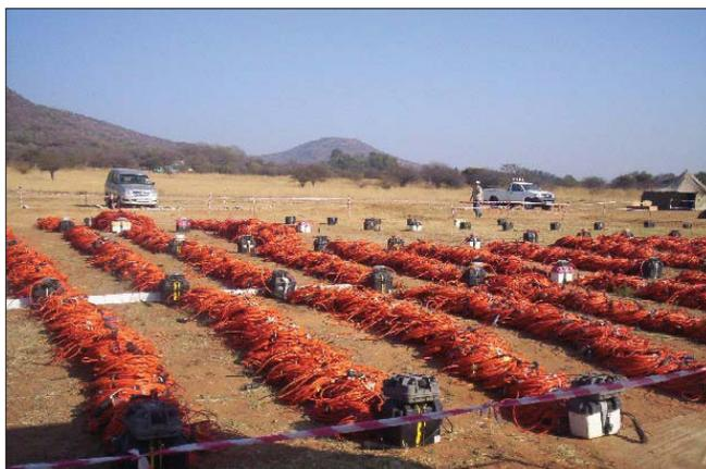
Figure 2. Land seismic acquisition system.
