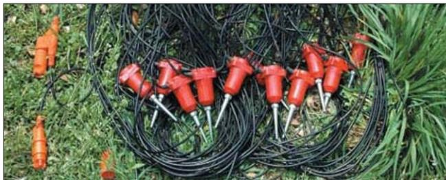
Figure 1. Geophone string with connectors.
